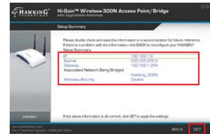
3.) The Setup Summary displays all your recently configured settings for the HWABN1 AP/Bridge. Please double check all settings to make sure they are correct and remember the IP address for logging into the web-user interface. Click 'SET' to apply all settings.
