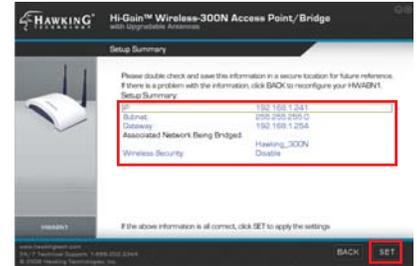
8.) The Setup Summary displays all your recently configured settings for the HWABN1 AP/Bridge. Please double check all settings to make sure they are correct and remember the IP address for logging into the web-user interface. Click 'SET' to apply all settings.
