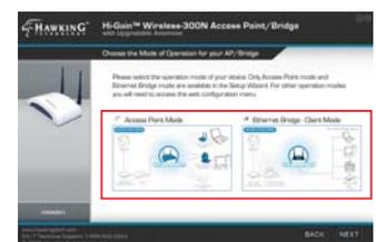
5.) Select an Operation Mode. Choose either Access Point Mode or Ethernet Bridge Mode. Click 'Next'. See Step 5a to continue operating in Access Point Mode or Step 5b to continue operating in Bridge Mode.
