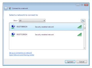
When the screen at left is displayed, select the network to connect to and click [Connect].
